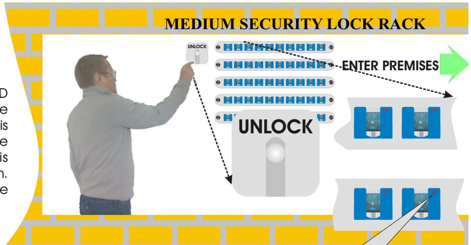
Red light indicates unlock status, the tag can be pulled from the rack
