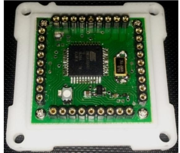
Hx7 I/O map: Pin numbers **1 - 44** correspond to the Atxmega 128A48, 64A4U/ 32A4U and 16A4U for further information go to [atmel.com](http://atmel.com) and view the datasheet for these micro controllers.
